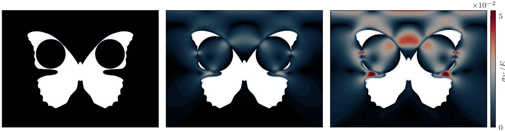
Figure 1: Development of Von Mises stresses for evolving deformable solids in contact. From the initial configuration, the disk is grown to introduce contact and, ultimately, stress, showcasing the applicability of our method to geometrically more intricate domains. Evolution from left to right, from a stress-free to a stressed system.
